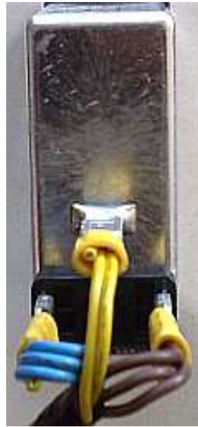
Figure 5-1(b): PEM's cables
