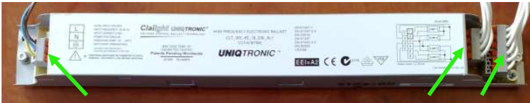
Figure 3-1: Electronic ballast wires (UNIQTTRONIC)
